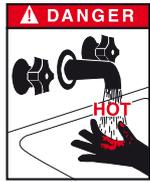
**The water which may flow out of the safety valve is very hot and may cause serious burns. The pipe discharging into the waste water disposal system should be open to the atmosphere. Make sure there is nobody near the flow of hot water.**
